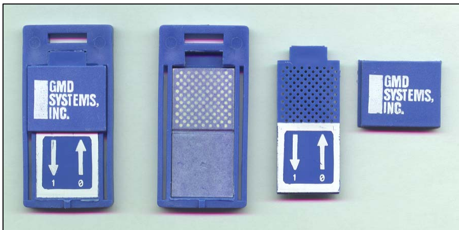
Figure 2: The GMD sampler with an exposed filter.
